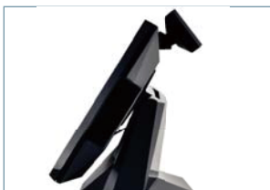
An ultra slim, fanless design to reduce the noise and prevent dust inside the unit
